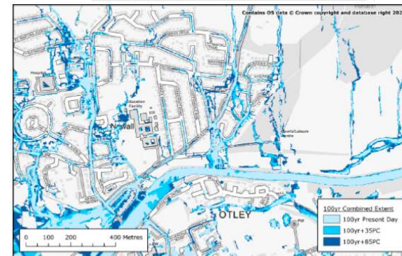
Figure 1-3: 100-year combined extent grid, Otley
